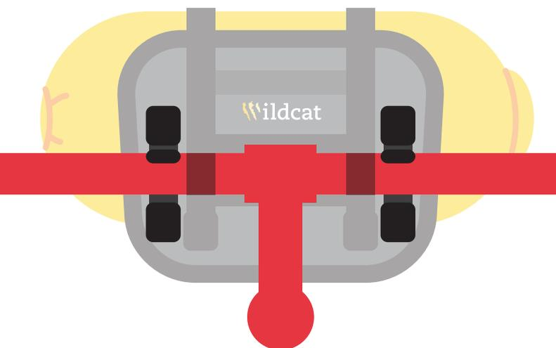
Place the Lioness retaining straps underneath the handlebar, just outboard of the Mountain Lion straps.
