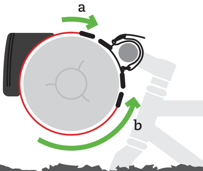
Place Lioness in position on the front of the dry bag and clip the top buckles of the Lioness into the retaining straps.
