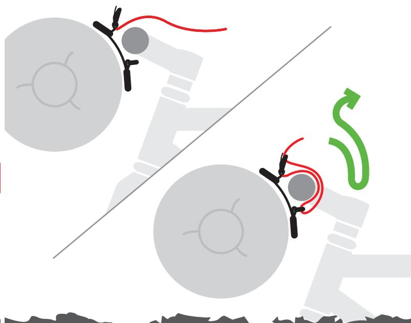
Take the free end of the strap and loop it over the top of the bar towards the rear. Thread it through the square loop and back over the top of the bar and through the camlock.
